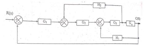
**Q.8** Find the overall transfer function of the system whose signal flow graph is [L5,CO1] 10M shown below.
