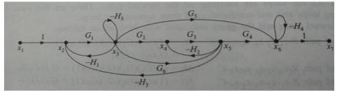
Using mason gain formula find the transfer function  $\frac{c}{R}$  for the signal flow [L3,CO1] 10M Q.10 graph shown in figure.
